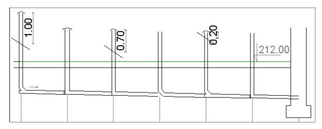
The "stack" object makes it possible to mark the stack and its horizontal branch on the longitudinal profile drawing. It can be especially useful during designing of sub-floor sewage systems. The user can define the following parameters of the object:
